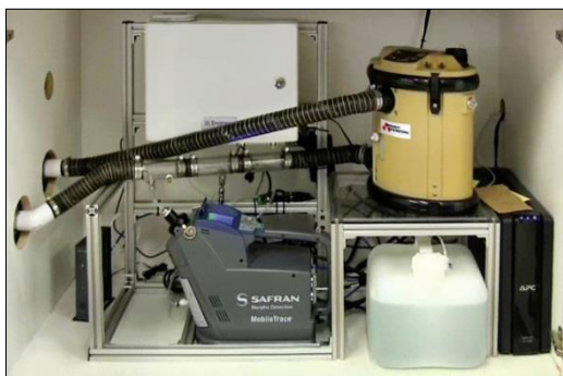
ASAP II System showing SASS 2300 air sampler with chemical detector and explosives detector.
