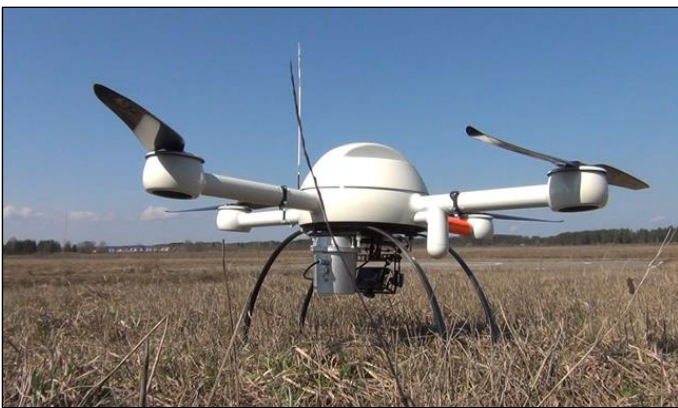
Figure 3: Radiation detector subsystem shown in a previous application, mounted in a cylindrical enclosure to the underside of a miniature UAV helicopter.
