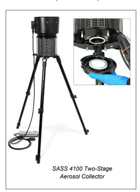
The SASS 4100 processes over 4000 liters/minute of ambient air that is continuously sampled as a primary air stream. Particulates in this air stream are transferred to a much smaller secondary stream using centrifugal and impaction principles. virtual Particles are then routed into the secondary flow by forcing primary circuit air to circulate through specially shaped channels where centrifugal force and particle momentum isolate and concentrate the particles. The
