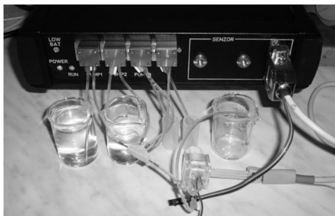
Fig. 3. Electrochemical device with four peristaltic pumps ( top ); flow-through cell with integrated reference electrode and screen-printed strip with four working electrodes ( bottom ).
