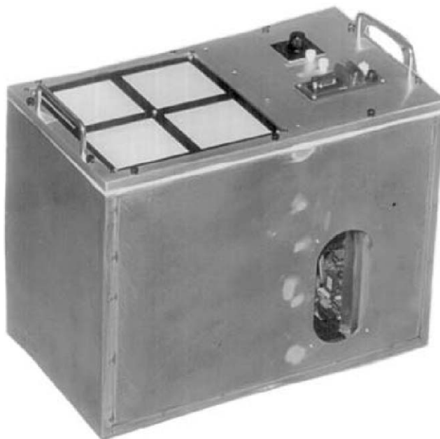
Fig. 6. Photograph of assembled RI-LLNL collector with virtual impactor inlet showing.
