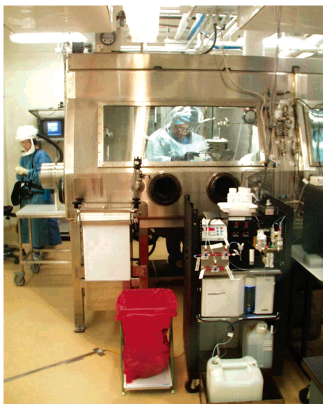
Figure 3. Biosafety-Level 3 containment aerosol chamber (CAC): The CAC is a stainless steel glovebox (5 m 3 ) with HEPA-filtered inlet and outlet air streams. The APDS can be seen in the foreground. The aerosol collector was removed from the chassis and placed inside the aerosol chamber. Aerosols of highly infectious anthrax spores and plague bacteria were generated using collision nebulizers. Aerosol particles were collected and concentrated in the aerosol collector and the aqueous sample pumped to the fluidics module for immunoassay processing and subsequent analysis.
