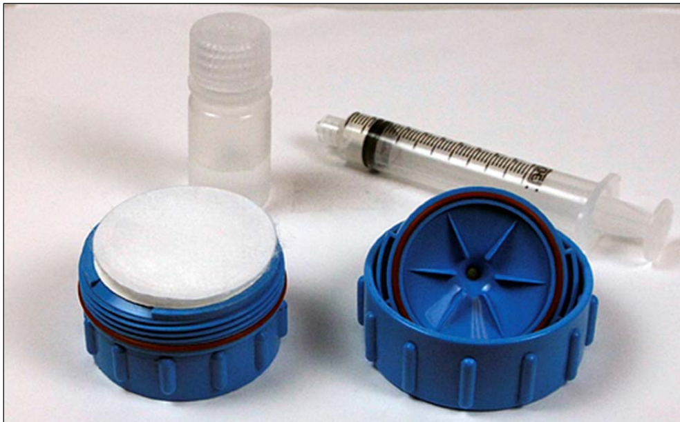
Figure 1: Opened 47-mm filter holder, syringe, and extraction fluid
