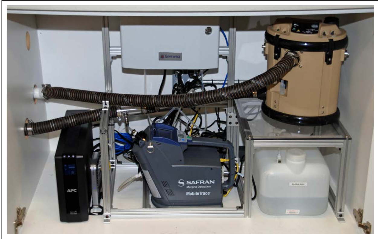
Figure 2: ASAP V postal room configuration with air sampler, chemical, and explosives nuclear detection.
