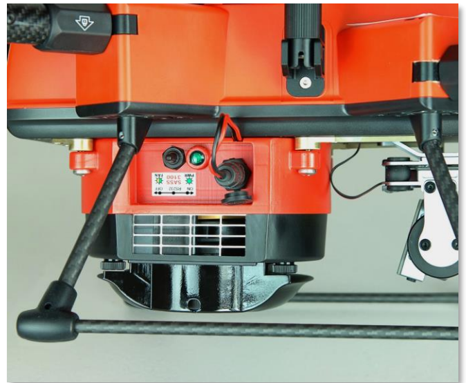
Research International air sampler mounted beneath drone
