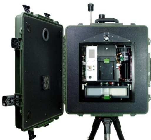
The TacBioHawk™ combines particle detection and bioidentification capability
