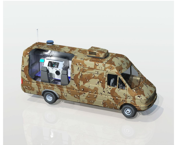
Figure 1. VBAD 3600 artist's rendering. The system is compatible with a wide range of vehicle interior spaces. Vehicle not included.
