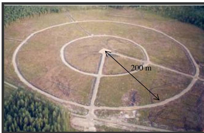
Figure 6. The region used for biological field trials located near the Swedish Defence Research Agency FOI, Umeå. The biological detection equipment is located in the center of the field. The release of the biological simulants takes place at a 100 or 200 m distance in radius from the equipment.
